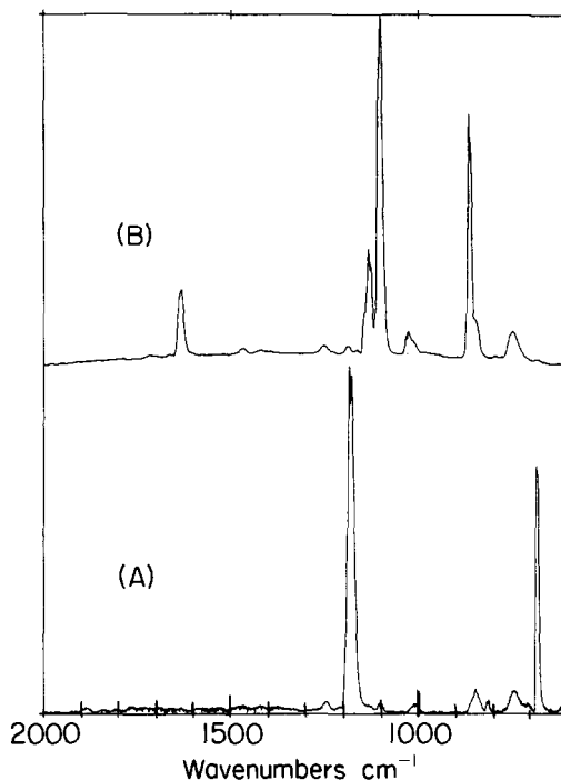
Fig. 1. Infrared absorbance spectra of (A) trans - and (B) cis -1,2-difluoro-1,2-di-iodoethene.
